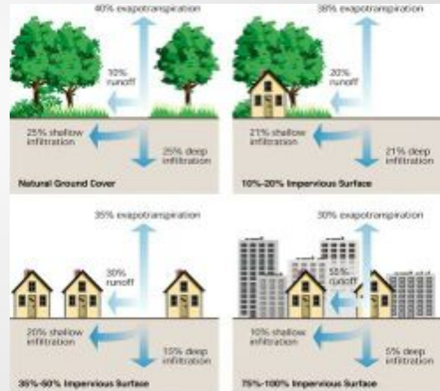
Fig. 2.21 - Relationship between impervious cover and hydrologic response. Impervious cover is a combined result of increased surface runoff. As little as 10 percent impervious cover is a combined run-off result in stream degradation. In Stream Corridor Evaluation: Principles, Processes, and Practices (2008). By the Federal Emergency Management Agency Working Group (FEMA) (2008) (2008) agency of the US.
